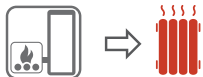
Central heating systems with one or more boilers which are plumbed together and do not generate domestic hot water.
