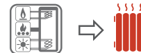
Heating systems with one or more sources hydraulically divided, with the exploitation of the solar power and without DHW production.
