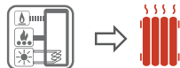
Central heating systems with one or more boilers which are plumbed together in conjunction with solar power which is connected to either one or two coil type heat exchangers. Domestic hot water is not generated in these tanks.
